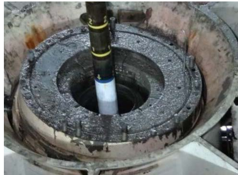
Lower half of failed LMRP Connector
