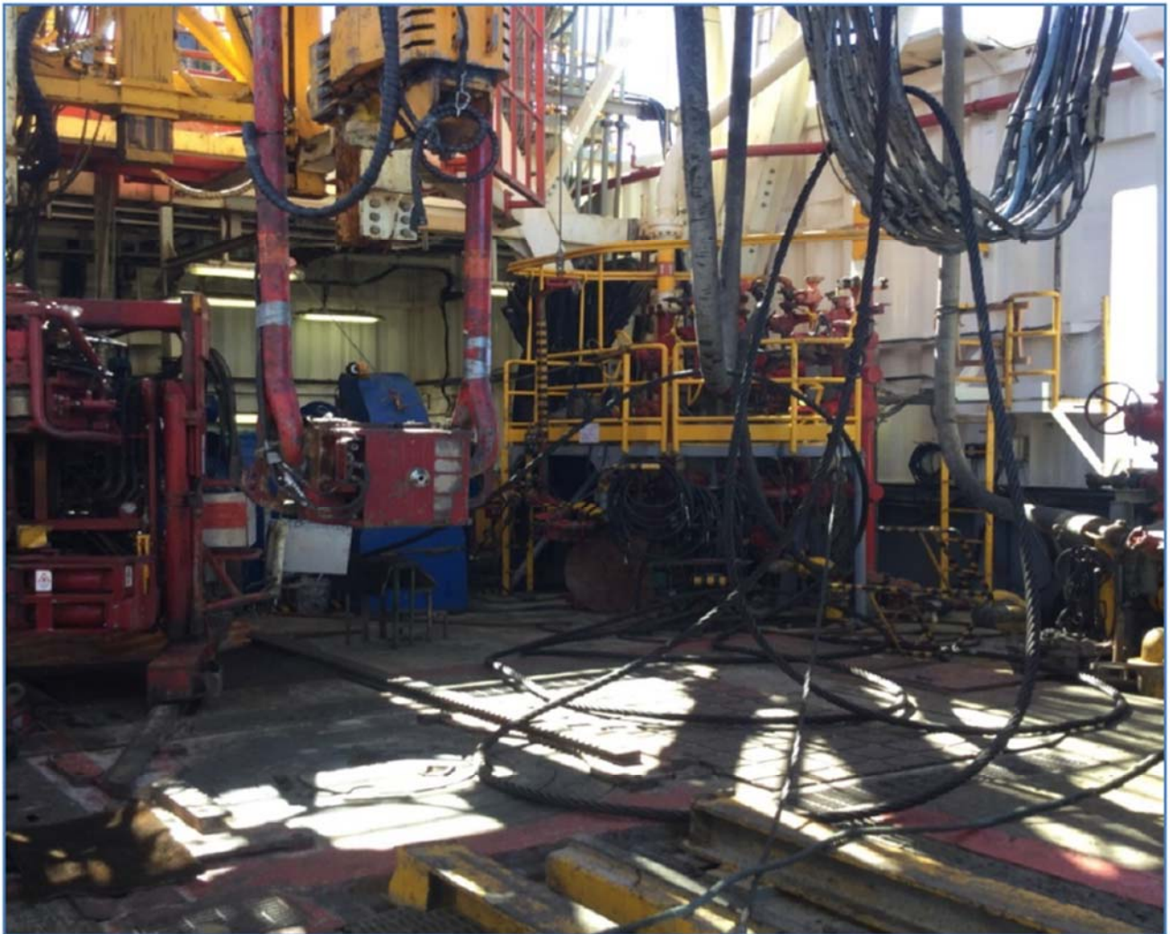
Drill line position after wire rope grip failed
