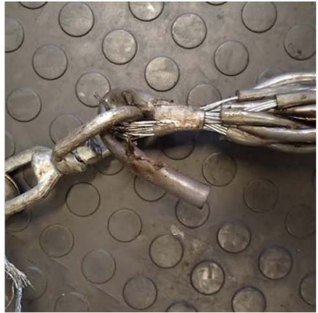
Failed components of the wire rope grip
