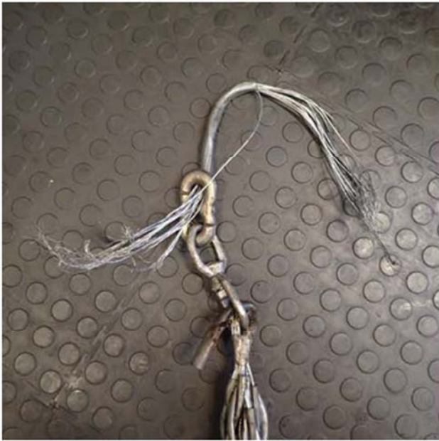
Failed components of the wire rope grip
