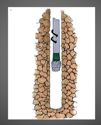
Punch In The Code On Your Surface Controller. Blow The Worn Tip Off the Drill String
