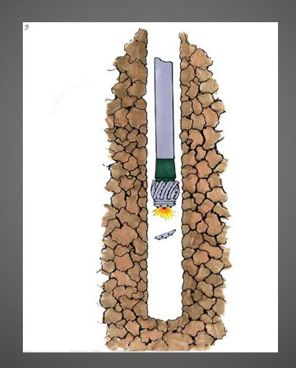
The Worn Tip Is Now Separated And Lies At The Bottom Of The Bore Hole
