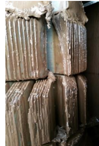
Evodos plate-pack loaded with oil-based mud solids
