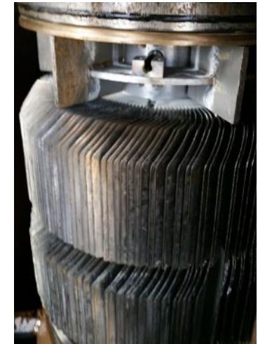
Evodos plate-pack after mechanical solids discharge
