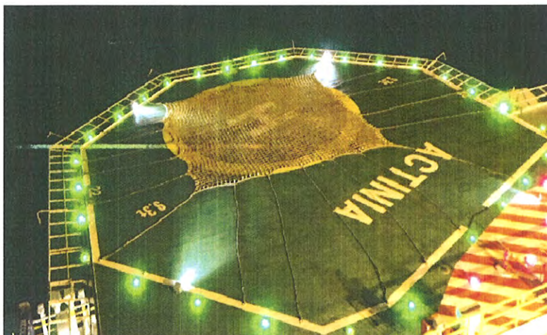
Picture of Helideck of Semi-Submersible MODU “Actinia” with Night Lighting:
