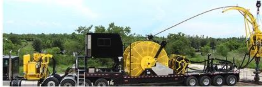
Coil Tubing Unit
