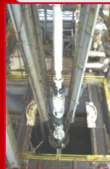
Concentric riser (DP) Above Tensioner Ring (US Patents 7,866,399 8,631,874)
