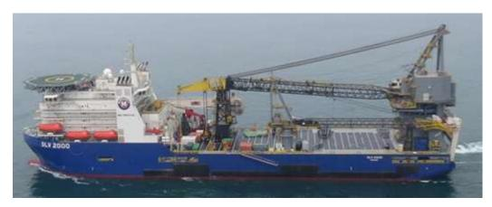
Figure 9 – Large conventional ship shape heavy lift vessel
