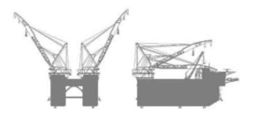
Heavy lift semi-submersible vessel
