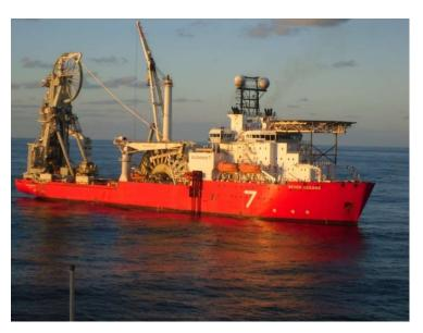
Figure 4 – Subsea 7's Seven Oceans pipelay vessel
