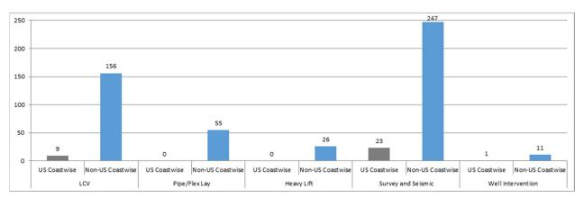
Figure 1 – Worldwide breakdown of deepwater OSV types (528 vessels)
