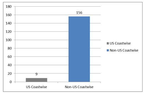
Figure 3 – Worldwide breakdown of deepwater capable light and medium construction vessels (>100T crane capacity; >1000m wire)
