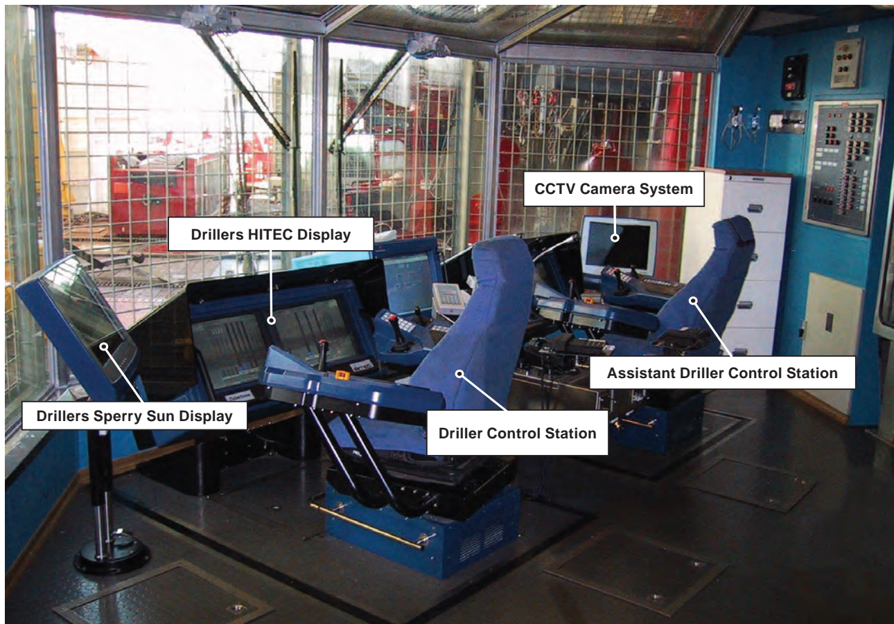
Figure 1 Deepwater Horizon Drilling Control Station
