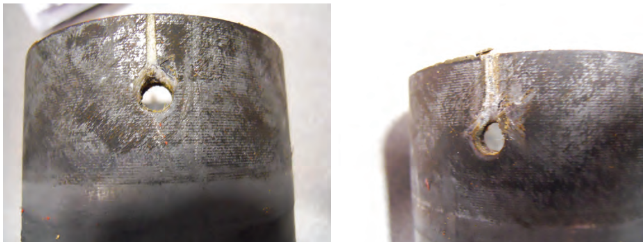
Figures 14 and 15 Flow Tube Damage During “Normal” Float Conversion Test
