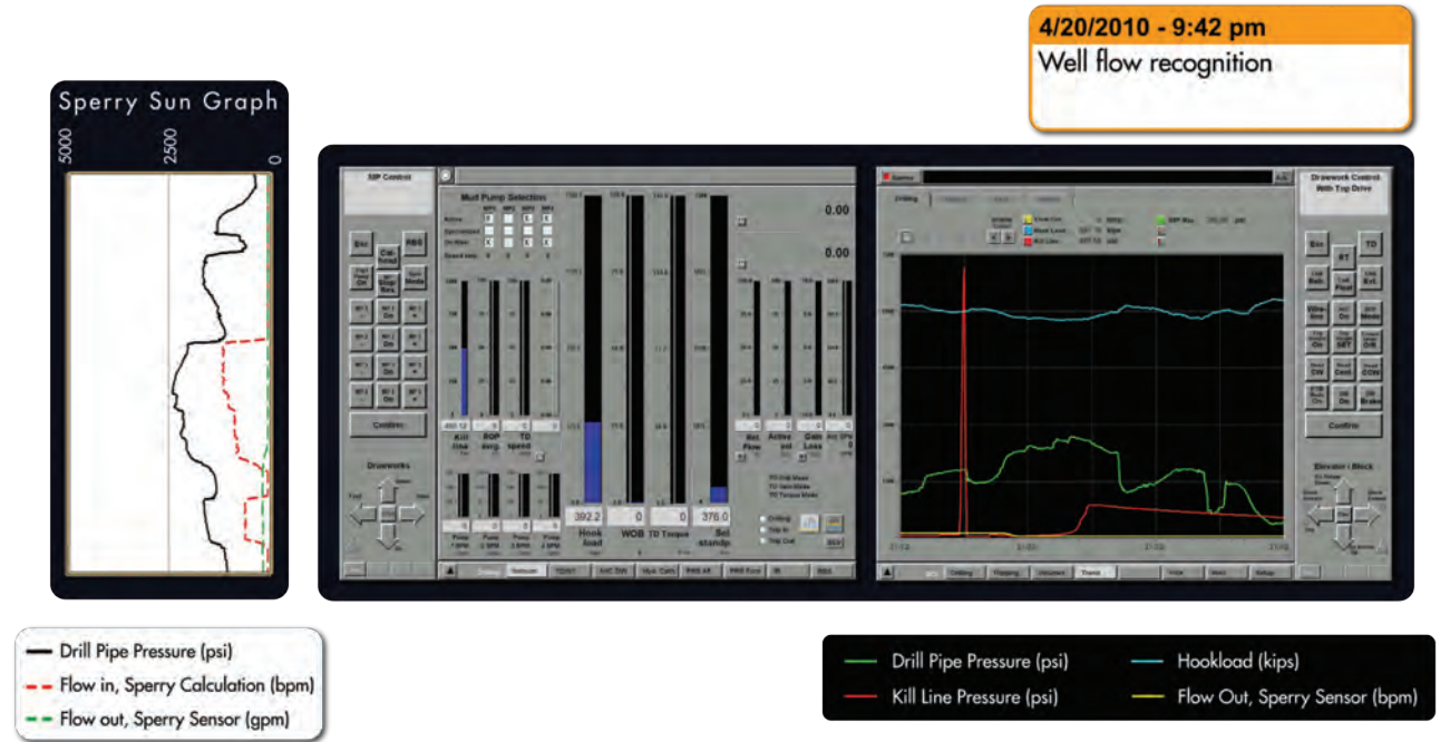
Figure 14 9:42 p.m. Trip Tank Fills
