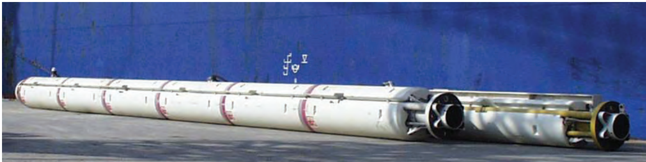
Figure 10 Deepwater Horizon ABB Vetco Gray Riser with Buoyancy Modules
