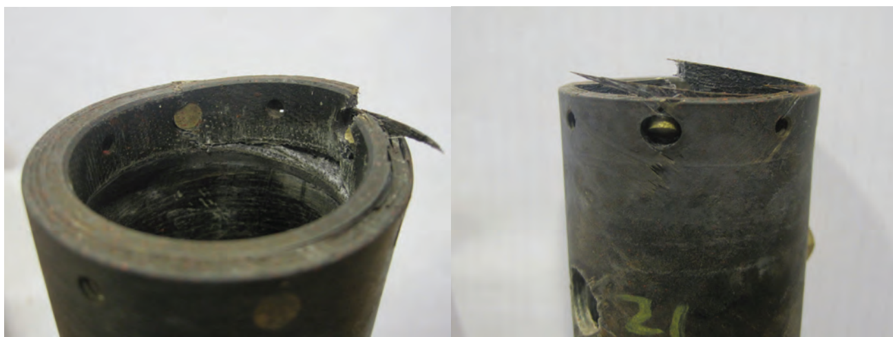
Figures 16 and 17 Actuation Ball Ejected Through Seat of Flow Tube
