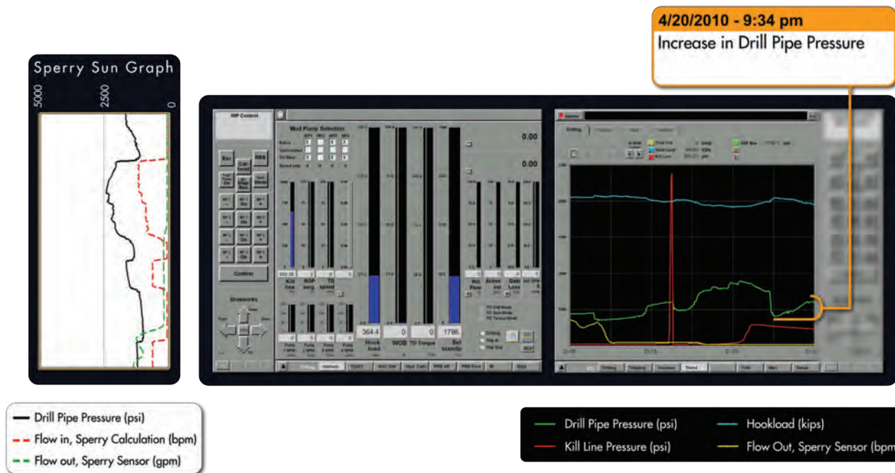
Figure 12 9:34 p.m. Pressure Increase With Pumps Offline
