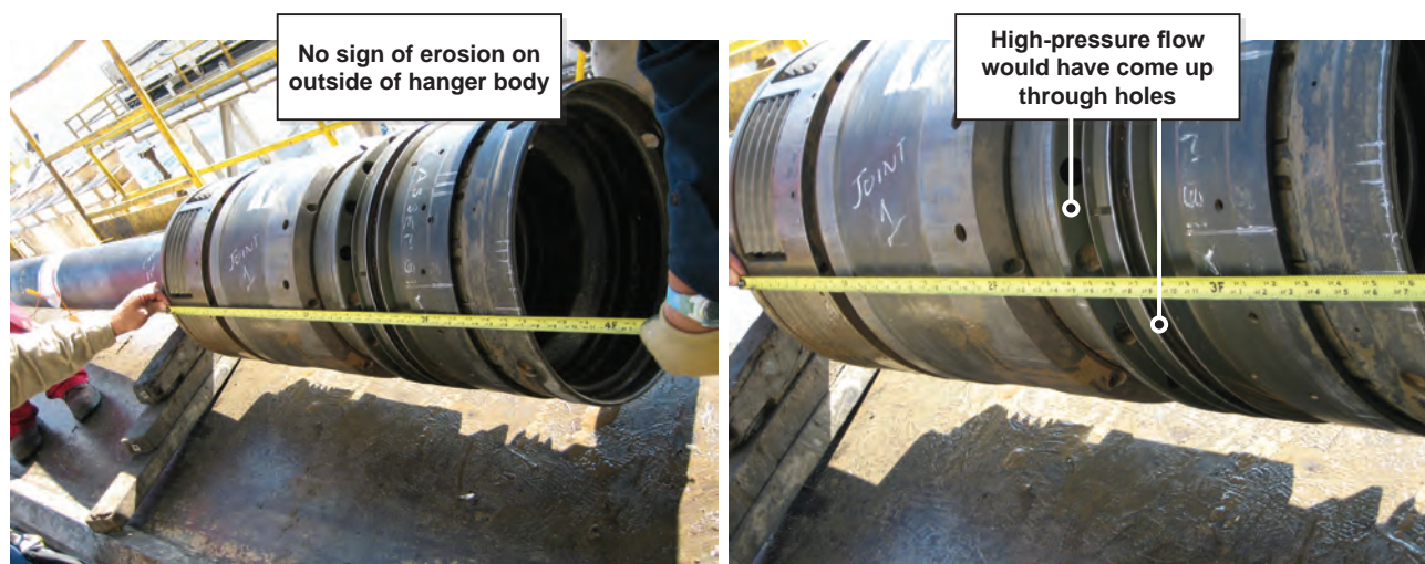
Figure 5 Macondo 9-7/8-in. Casing Hanger (Exterior)
