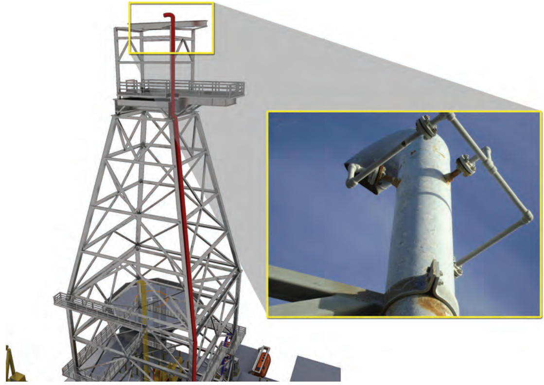
Figure 3 MGS 12-in. Vent Line at the Derrick Crown
