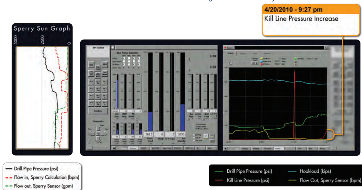
Figure 10 9:27 p.m. Kill Line Pressure Climbs to 833 psi.
