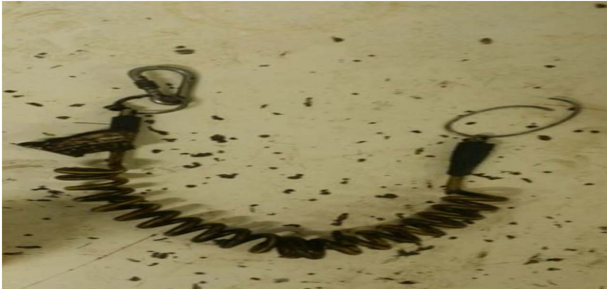
Tool lanyard with broken ring
