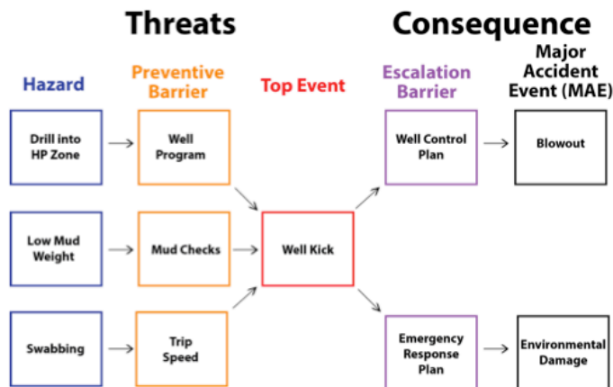
Example Bow-Tie analysis diagram for a well kick while drilling
