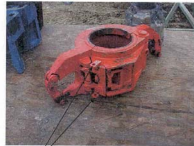
Note: The elevator has the tabs installed as per manufacturer's specification but the safety latch lock pin and safety chain had been removed.
