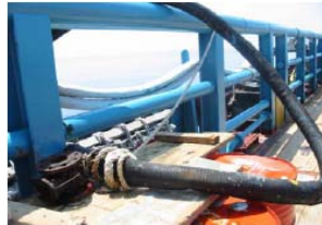
Hose with valve and chain attached after whipping out of the sea
