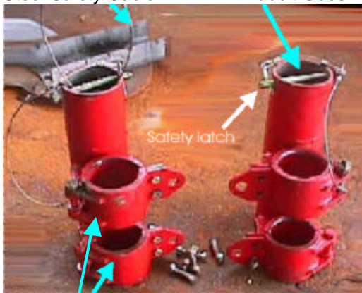
Two Clamps that attach the Rabbit Carrier to the Bails.
