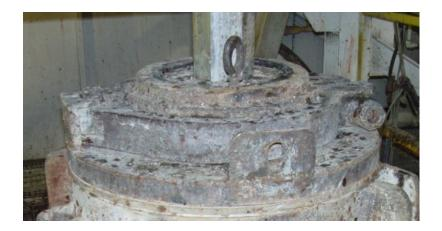
On this model of rotating control device, the entire clamp assembly rotates along with the kelly. SRL line apparently became entangled in some portion of the clamp assembly.
