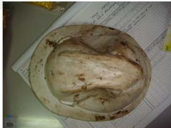
Photo 3 damage to Hard Hat
