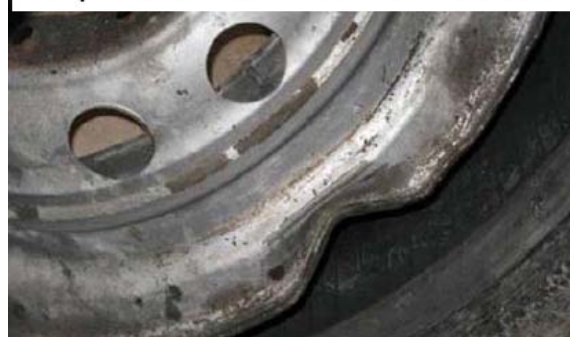
Inside edge of the wheel rim indicating impact when it struck the roof cross-beam
