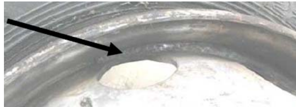
Weld area from hub side
