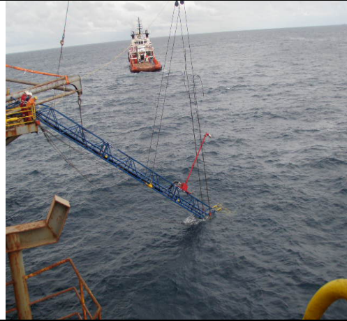
Starboard Boom After Failure
