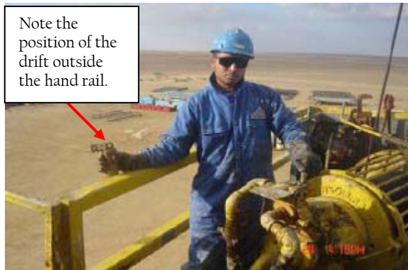
The position of the floor man before the drift slipped from his right hand.
