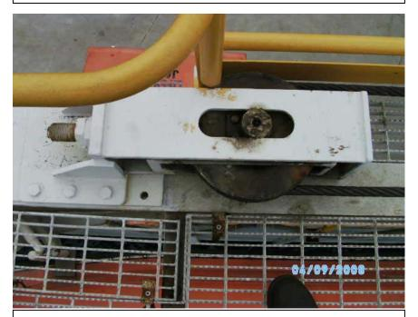
View of adjusting sheave with housing designed to catch/hold sheave in the event failure. Engineering will assist Operations with upgrading open sheaves to this enclosed type.
