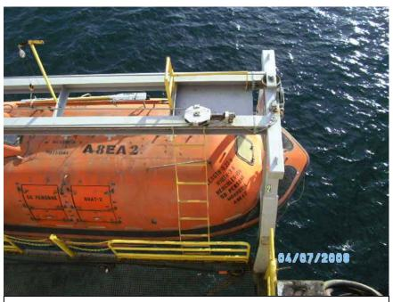
View of open type adjusting sheave without housing that will not catch/hold sheave in the event of failure.
