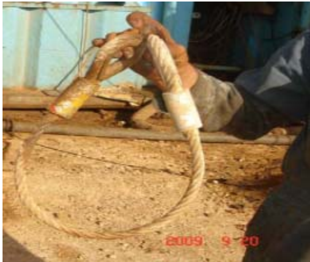
Wire rope sling that dropped to the rig floor.
