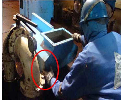
The IP's hand position between the air duct and pipe flange
