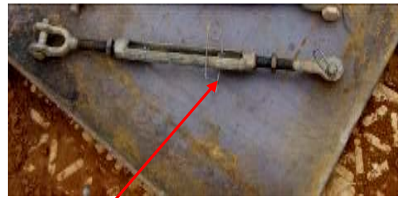
Safety pin fitted to inside thread end
