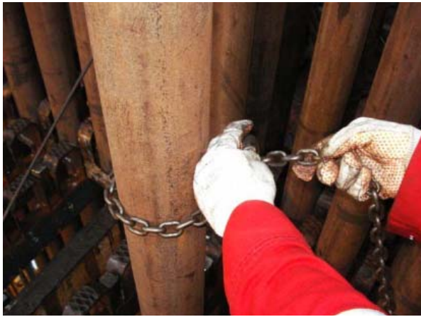
Demonstrating placing the chain on the stand of pipe.
