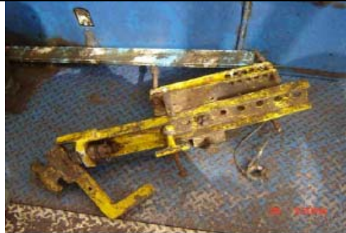
The intermediate tieback (Approx. 12kg) was fell from 10 meter height to the rig floor
