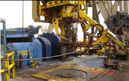
The make – up tong was used to hold the lower IBOP while they torque the upper IBOP in the reverse direction
