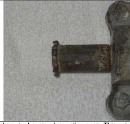
Speaker wire housing / mounting post. This point was flush with the junction box where it broke loose.
