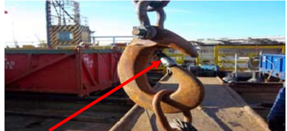
New Locking Mechanism In Place As A Result Of Incident
