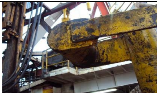
Starboard V-Door King Post with identical pipe. (This was removed after the incident.)
