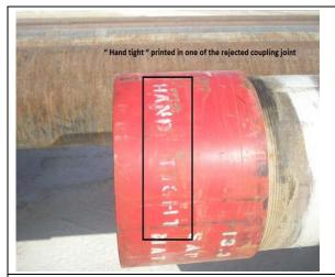
"Hand Tight" printed on the coupling of a rejected casing joint.
