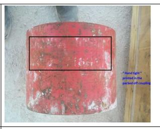
"Hand Tight" printed on the backed off coupling joint.
