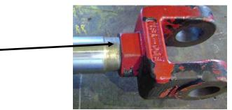
The clevis was removed from the replaced extender cylinder assembly and was taken out of service for inspection and galling of the threads was discovered. This leads to the conclusion that if there is a gap between the shoulder of the shaft and the clevis, there is potential for failure and injury.
