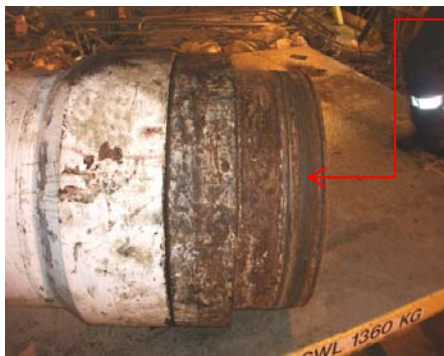
Condition of threads on parted diverter
