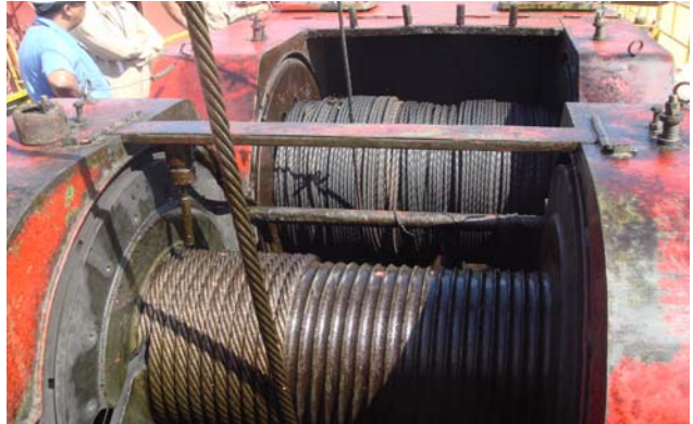
View of drawworks drum and sand-line drum
