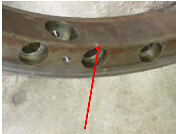
Cracked Wall in Ring:
