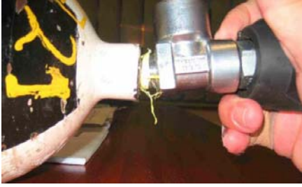
Valve alignment with BA bottle and bent valve under rubber cap
