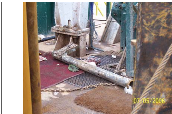
Photo 1 – Slide Bar after falling to rig floor
