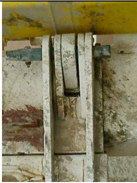
View showing that one pin held both the grating and the finger assembly.
