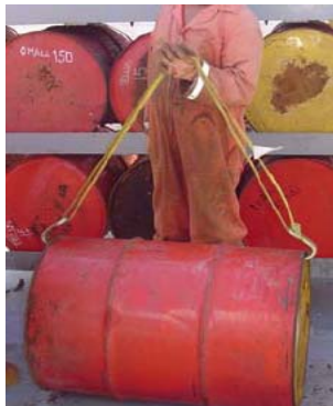
Figure # 3 Incorrect attachment
