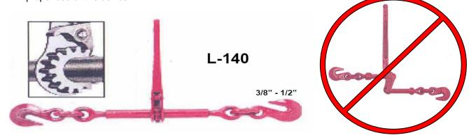
IADC Note: Lever binder manufacturing companies recommendation against use of cheater pipes when either closing of opening lever binders.
